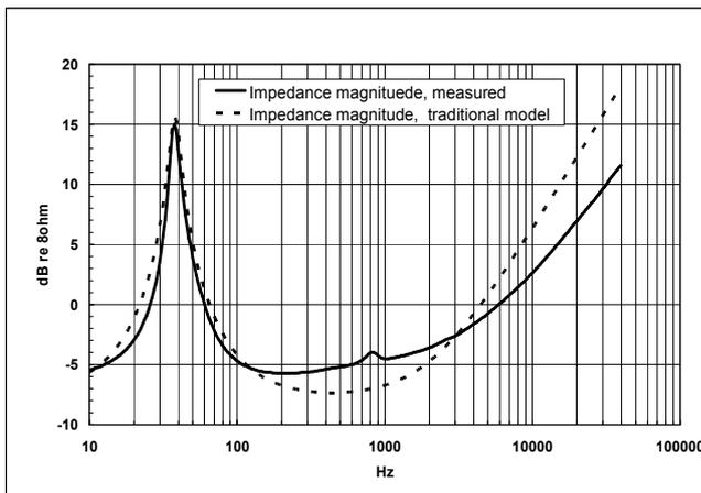
Fig. 3. Loudspeaker impedance measured and simulated according to the traditional model
