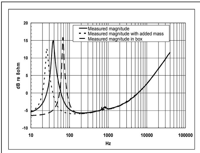
Fig.6. Loudspeaker impedance measured in free field (solid) and to the left (dashed) with mass added to the cone and to the right (dash-dot) mounted in an empty box
