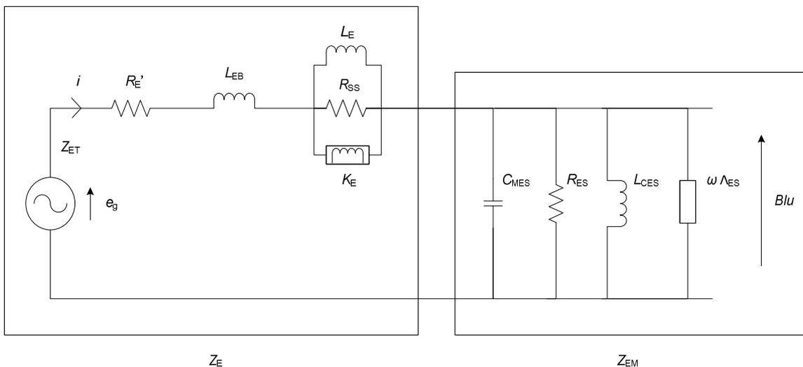
Fig. 7. The FDD/semi-induction model for the dynamic loudspeaker
