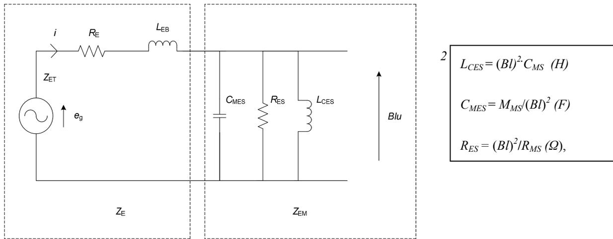
Fig. 2. The model Fig. 1 converted to the electrical side
