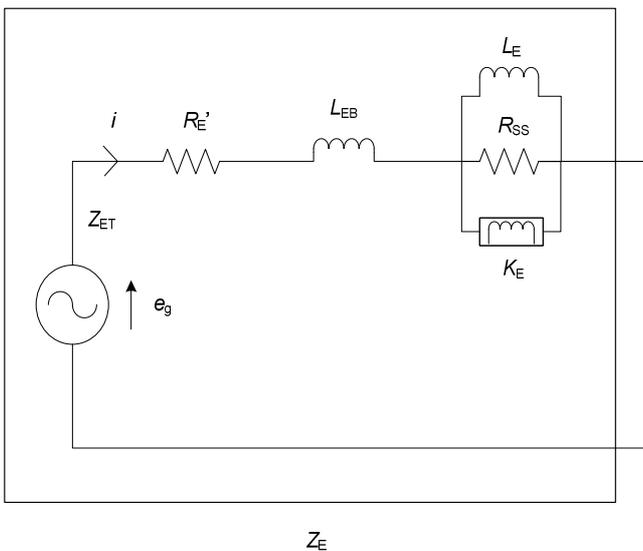
$R_E'$  substitutes  $R_E$  and includes additions due to eddy currents in “ac-shortening devices” outside the air gap.
