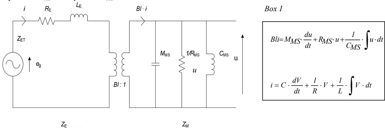
Fig.1. Traditional model for the dynamic loudspeaker according to the “admittance analogy”
