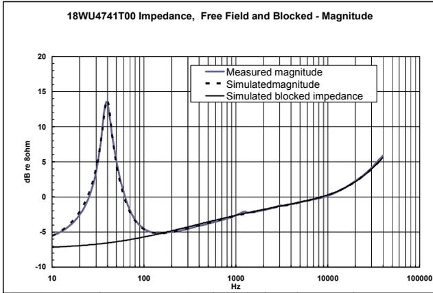
Fig. 8. Impedance, magnitude simulated according to the FDD model to the measured curve
